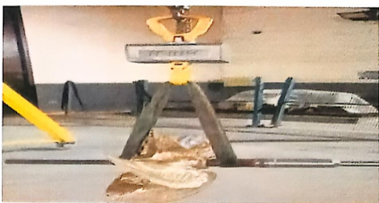
WEIGHT OF FIXED PROPELLER SHOWN ON SCREEN 104KG (WITHIN TOLERANCE)
